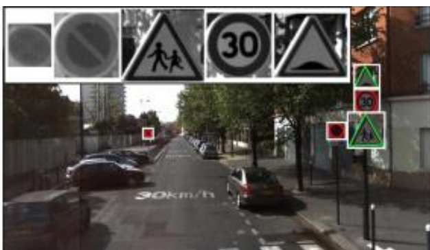
Fig 3.1. An example of using contour fitting to detect road signs within an image. [6]
