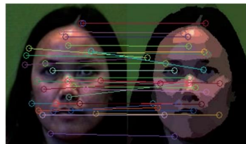
Fig 1.2 Example of SIFT extracted features showing the correlations between the original image and a processed eigen face image. [2]
